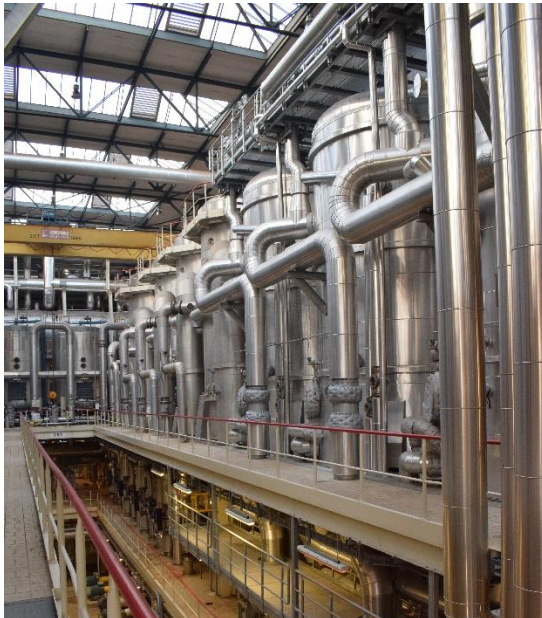
Foto 1: Cosun Beet Company: meertraps indamping
